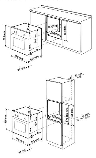
In order to ensure adequate ventilation, the back panel of the cabinet unit must be removed. Installing the oven so that it rests on two strips of wood is preferable. If the oven rests on a continuous, flat surface, there must be an aperture of at least  $45 \times 560$  mm.
